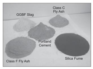
cementitious properties by itself but these are enhanced when it is used with portland cement. Slag is used at 20% to 70% by mass of the cementitious materials.
