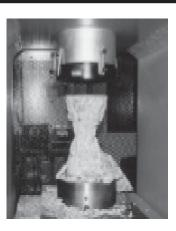
No single strength test should fall below f' by more than 500 psi (3.45 MPa); or by more than 0.10 f' when f' is more than 5000 psi (35 MPa)
